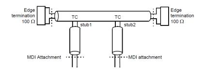
Figure 168–17—Mixing segment and reference points
