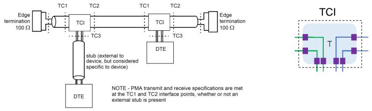
Figure 168-17-Mixing segment and reference points
