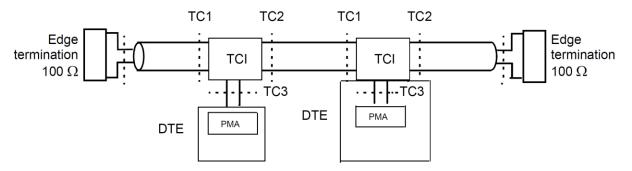
NOTE - PMA transmit and receive specifications are met at the TC1 and TC2 interface points.
