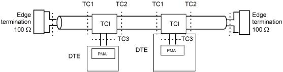
NOTE - PMA transmit and receive specifications are met at the TC1 and TC2 interface points.
