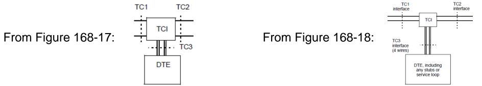
But, simulations and return loss specification use a 2 wire interface
