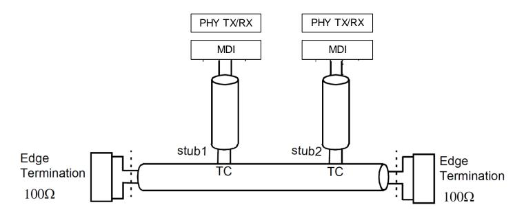
**1.4.403 mixing segment:** A medium that may be connected to more than two Medium Dependent Interfaces (MDIs).
