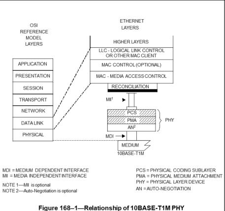
Figure 168–1—Relationship of 10BASE-T1M PHY to the ISO/IEC OSI reference model and the IEEE 802.3 Ethernet model
