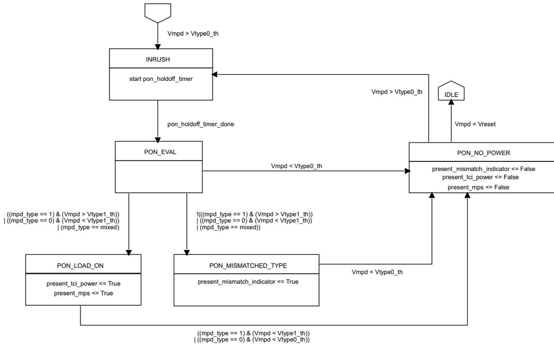
Figure 169-76 - Top Level PD state diagram (continued)
