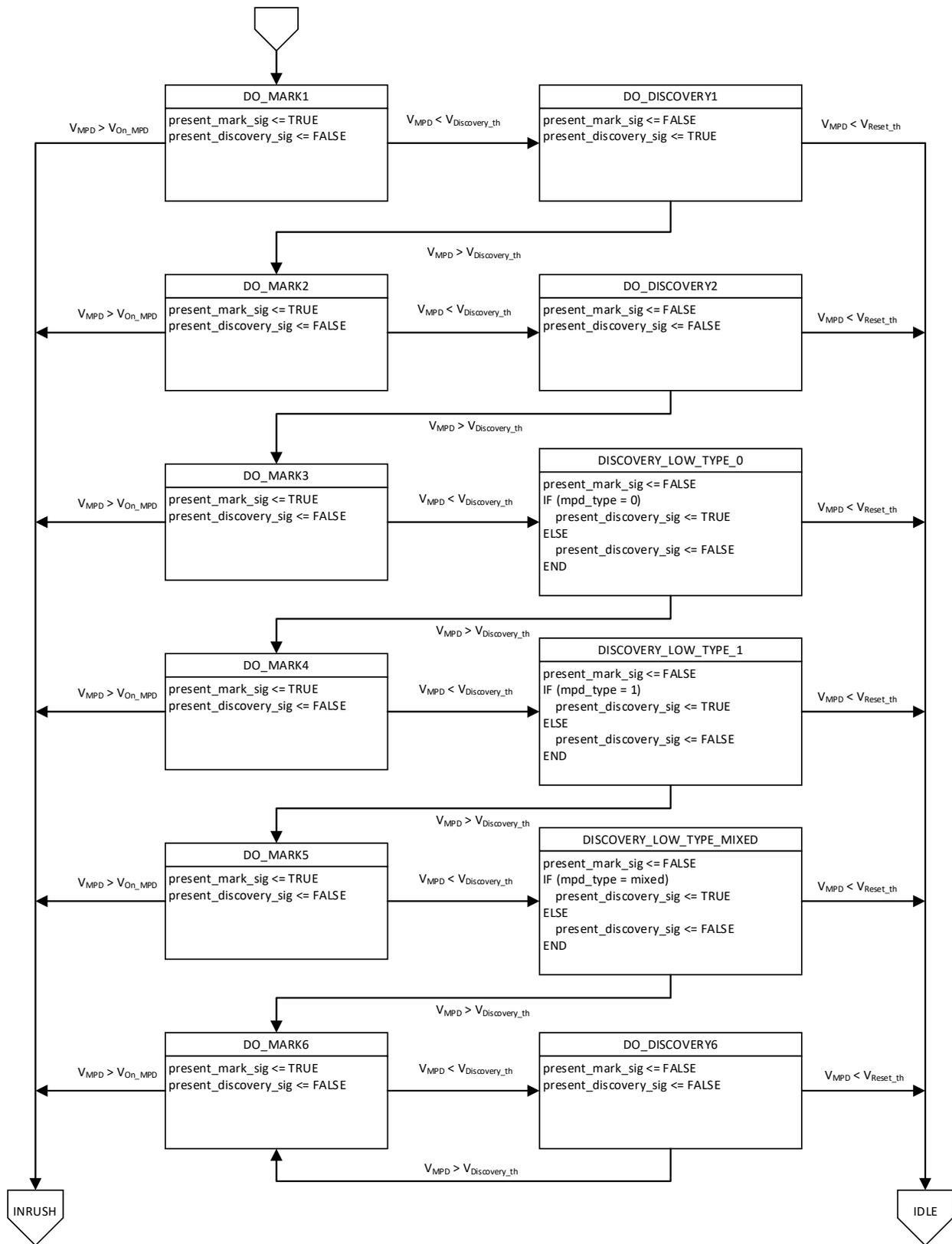
Figure 169-65 - Top level PD state diagram (continued)
