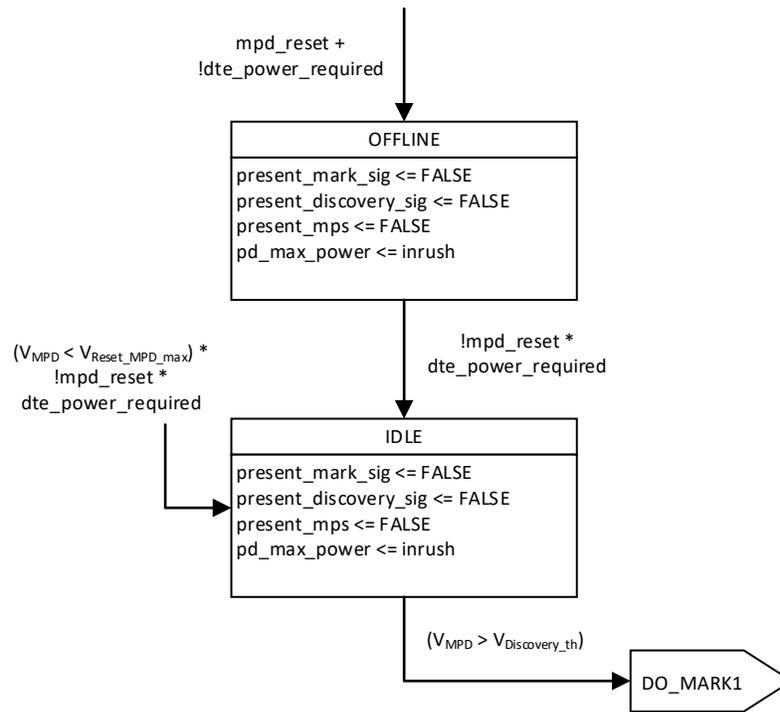
Figure 169-54 - Top level PD state diagram
