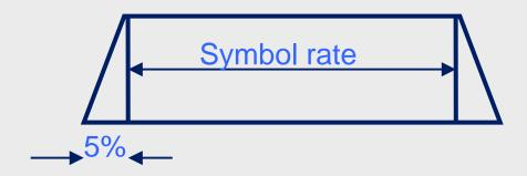
■ With new QAM filter-less designs, the total overhead goes down to 10% since no guard band is required.
