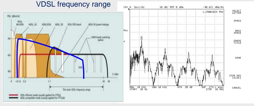
QAM rate adaptive algorithm detects the noise and shifts the carrier frequency and symbol rate to work around the T-LAN
