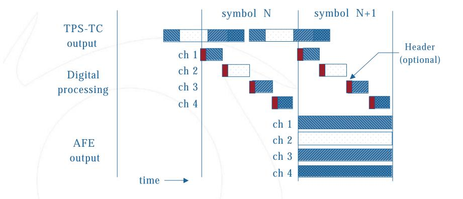
Data flow thru 4 channel Bonded DSL system
