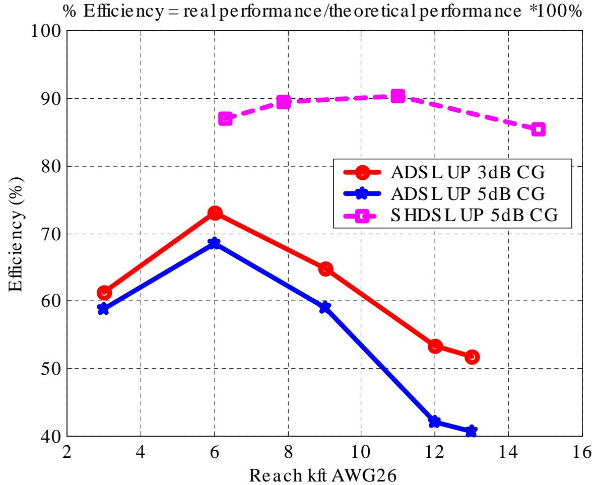
*There is a significant gap for ADSL between theory and performance testing.
