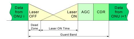
Figure 2: Structure of the guard band.
