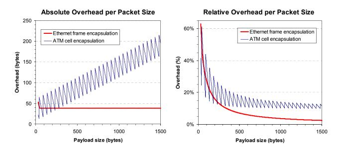
Figure 1: Comparison of Ethernet framing overhead and ATM cell tax.
