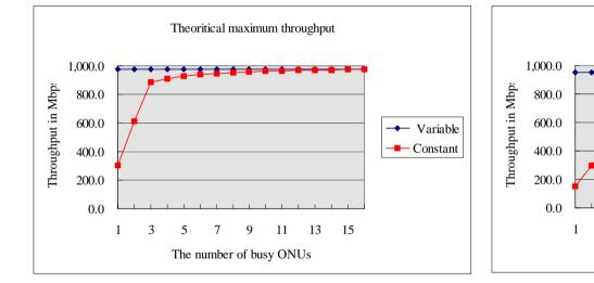
Guard time = 1.0 usec Maximum cycle time = 1.0 msec RTT = 200usec Line rate = 1,000Mbps Length of report message = 64Byte Max number of ONUs = 16 Guard time = 1.0 usec Maximum cycle time = 1.0 msec RTT = 200usec Line rate = 1,000Mbps Length of report message = 64Byte Max number of ONUs = 32
