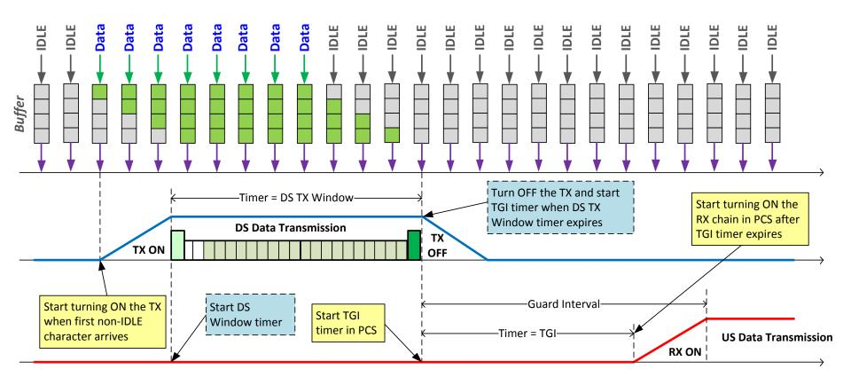
Data detector to command TX ON at the CLT – TX ends with configured delay after TX gets ON (DS TX Window, configured) and then RX starts with configured delay after the transmitter is OFF (TDD Guard interval, depending on max RTT)
