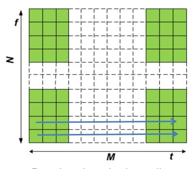
Data is written horizontally subcarrier by subcarrier to allow time interleaving of codewords
