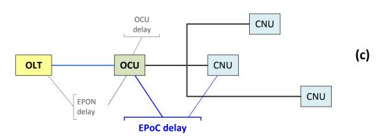
Similarly, the case of EPON with digital fiber can be easily considered adding EPON delay and OCU delay terms.
