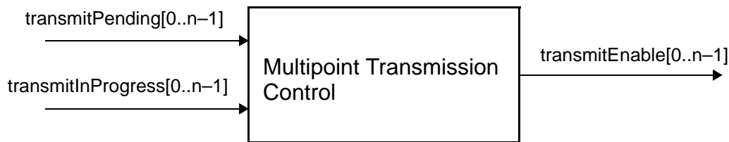
Figure 102-6—Multipoint Transmission Control service interfaces
