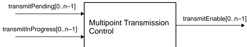
Figure 4-6—Multipoint Transmission Control service interfaces
