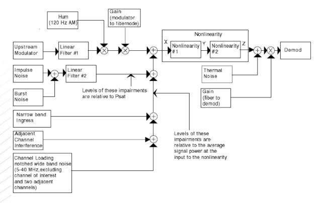
Figure 1. Upstream HFC Impairment Model Block Diagram
