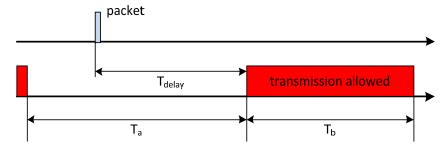
No increase of jitter (all packets will have maximal delay)
