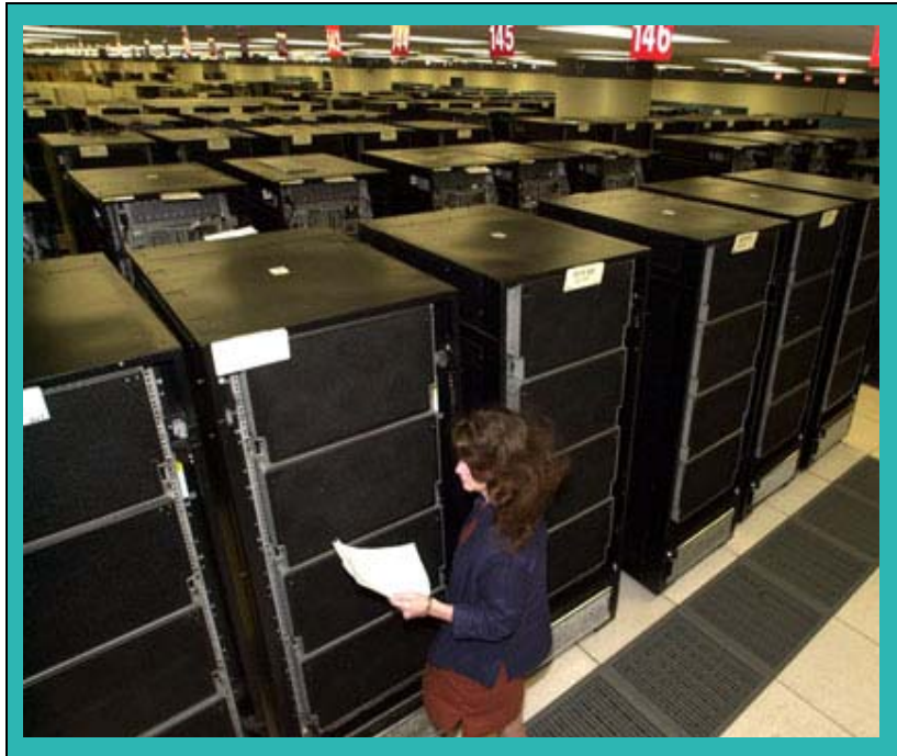
IBM ASCI Purple Server (LLNL) 75.7 TeraFLOP/s, ~3000 parallel links 12+12@2.5Gb/s/ch
