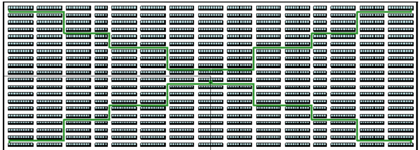
200' x 500' Datacenter w/ 2800 Racks or Cabinets (100m covers any-to-middle in this sized datacenter)
