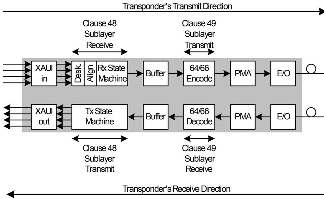
It should be made clear that clause 48 “receive” direction always corresponds to data incoming from XAUI (although might be called the transponder’s transmit direction) while the “transmit” direction corresponds to data sent to XAUI (which might be called the transponder’s receive direction).
