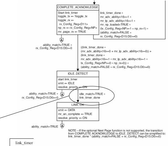
Timer used to ensure Auto-Negotiation protocol stability and register read/write by the management interface.
