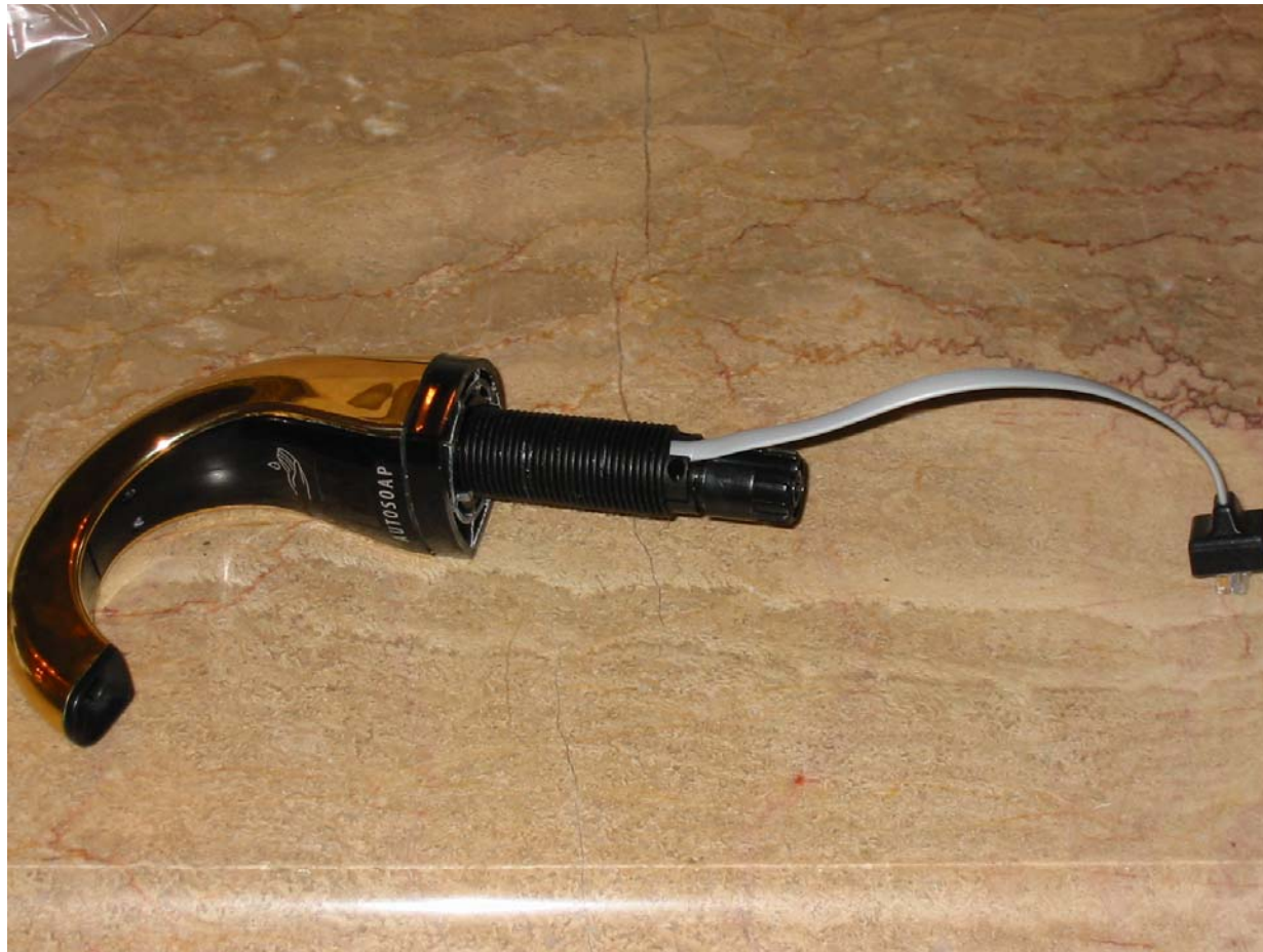
The Ethernet/802.3af Powered soap dispenser
