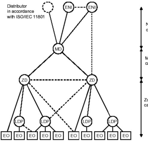
Network access cabling subsystem
