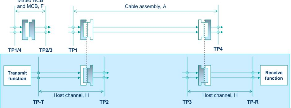
NOTE 1 – Only one direction of transmission shown NOTE 2 – Channel insertion loss is  $C = A + 2 \times (H - F)$
