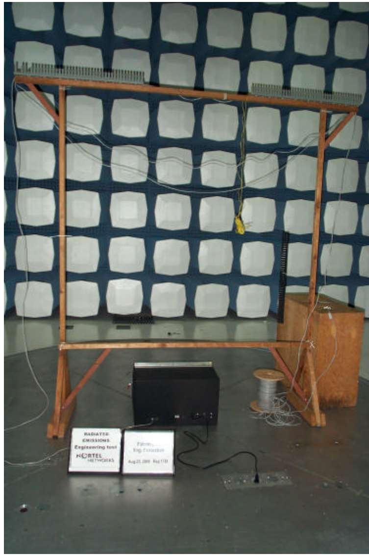
picture of Faraday cage, and UTP loops
