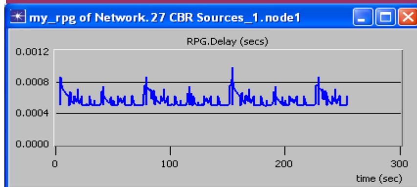
❑ 27 CBR Sources\_1, 9 CBR Sources\_1 subnet, node 4 to node 1, rate offset by -10 ppm
