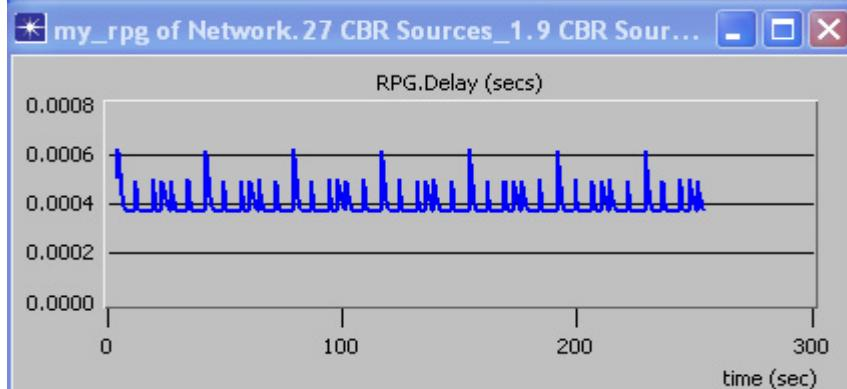
❑ 27 CBR Sources\_1, 9 CBR Sources\_1 subnet, node 5 to node 16, rate offset by -50 ppm
