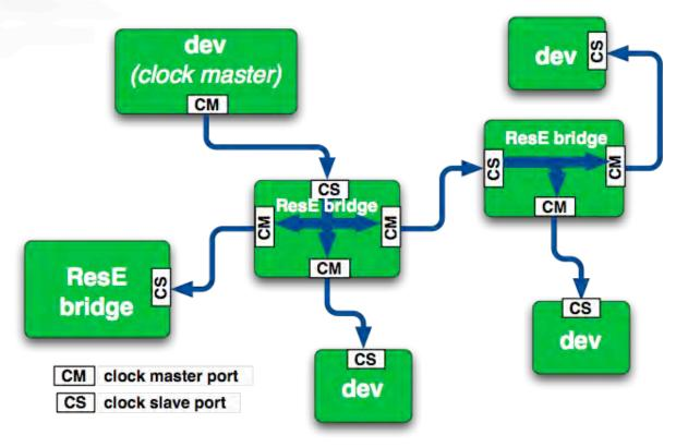
There is a single device within a ResE "cloud" that provides a master timing signal.
