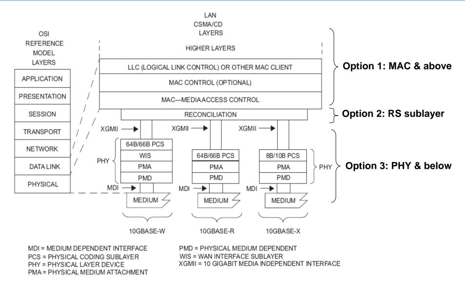
Figure 44–1—Architectural positioning of 10 Gigabit Ethernet
