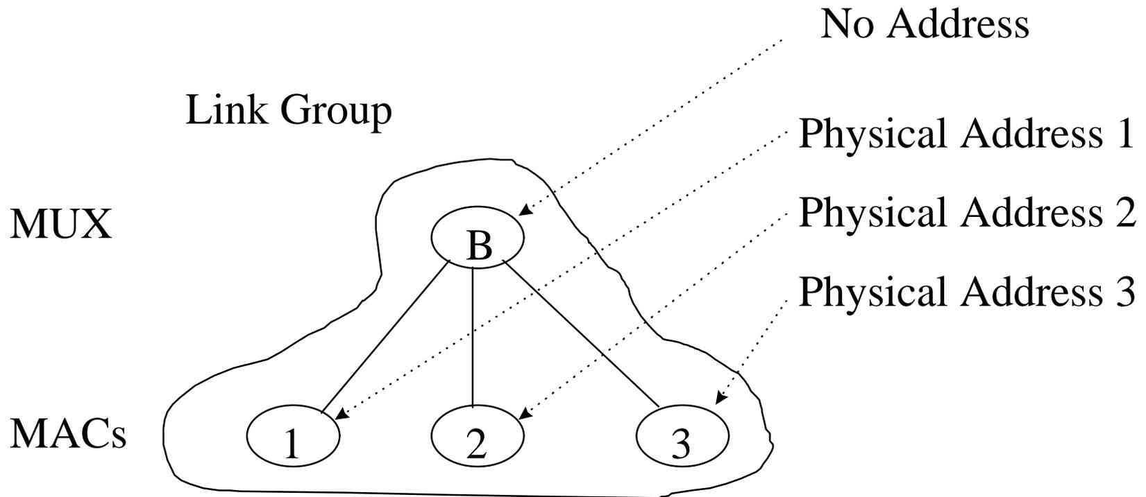
Bridge Uses Physical Addresses to source BPDUs etc.
