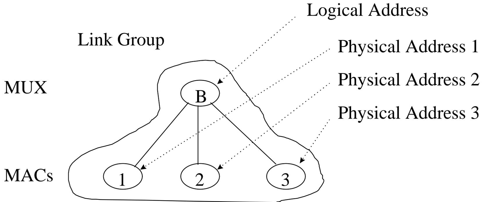
MACs either pass SA from MUX or generate SA with Physical Address
