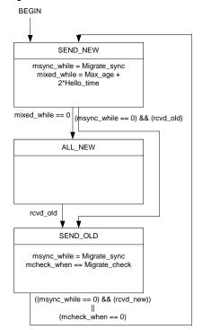
In the all new state the initial value of fd\_while assigned in the DBT and DLT states (see the state machines proposed in P802.1w/D2) can be cut to Hello\_time.
