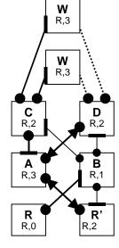
A receives message from C first (arbitrary), chooses A-C as new root and forwards message to D and R'. Ws receive messages from C and D without change.
