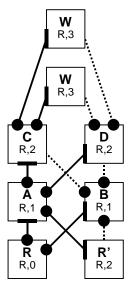
Spanning tree links (solid), redundant links (dashed). Configuration: <root>,,<root path cost> Black blobs indicate designated bridge for link. Short black line indicates root port.
