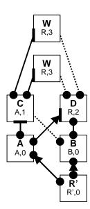
D receives from B, becomes designated on D-B. C receives from B, moves root port to C-A with A as root. R' receives from B and becomes root, transmits on R'-A and R'-B.
