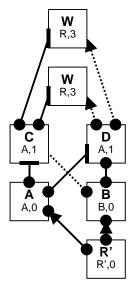
D receives from A, recognizes A as root and transmits to Ws.
