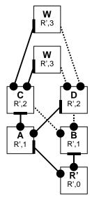
Ws receive messages and adopt R' as root. C and D receive message from A and select C-A and D-A as root ports. Messages will be forwarded to Ws, but final configuration has been reached.
