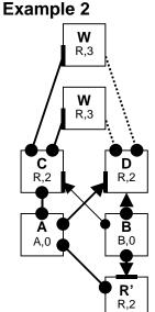
Many possible next steps depending on order of processing of messages in transit. Say C receives from A first and moves root port to C-B. Similarly R' receives from A and moves root port to R'-B.
