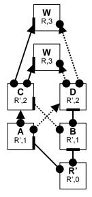
Assuming C and receive from B first, they acknowledge R' as root, selecting C-B and D-B as root ports.and transmit to Ws,
