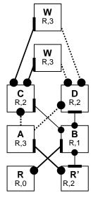
A receives messages from R' and D, moves root port to A-R' and transitions A-C and A-D to Blocking. D and R' discard messages from A.
