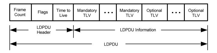
Figure 8.3 LDPDU header
