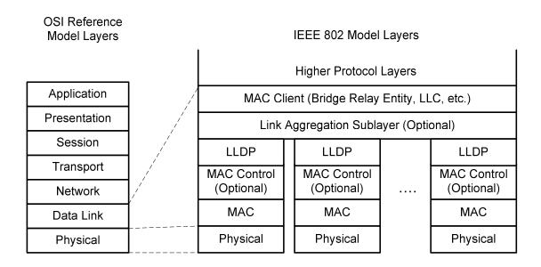
Figure 6.1 Architectural positioning of LLDP
