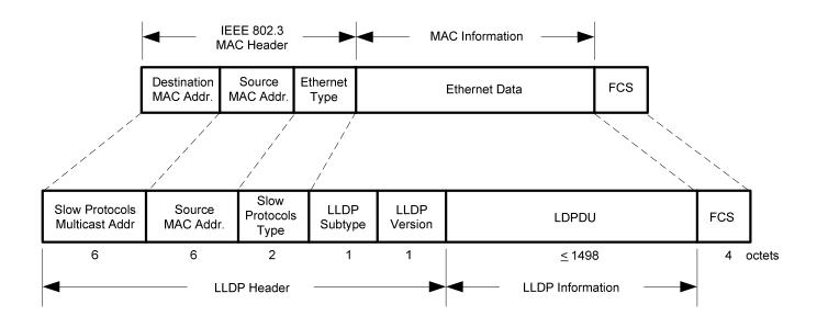
Figure 8.1 802.3-based LLDP frame format
