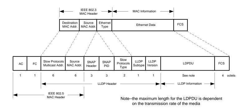
Figure 8.2 802.5-based frame format
