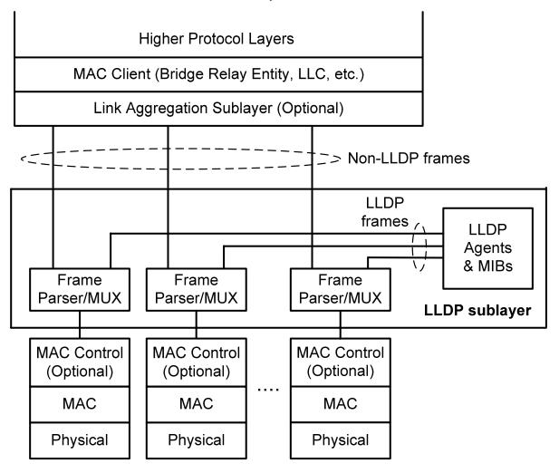
Figure 7.1 LLDP frame multiplexing
