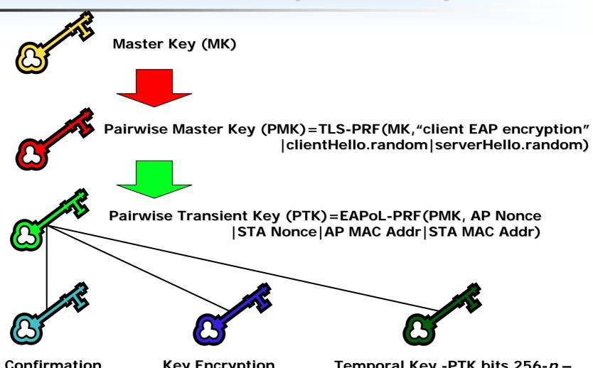
Key Confirmation Key (KCK)-PTK bits 0-127 Key Encryption Key (KEK)-PTK bits 128-255 Temporal Key -PTK bits 256-*n* – can have cipher suite specific structure
