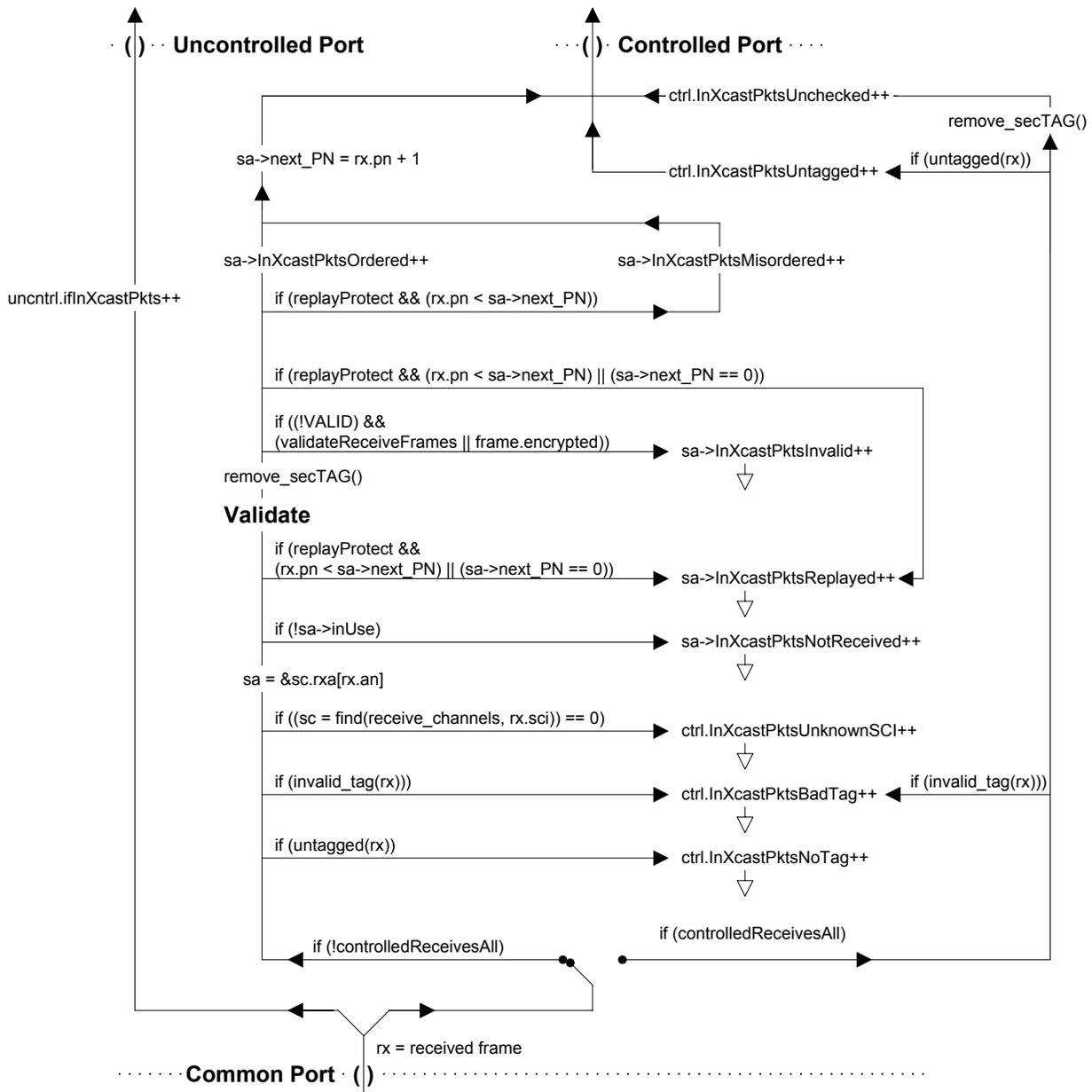
NOTE-- the notation xxXcastPktsxx++ means increment xxUcastPktsxx, xxMulticastPktsxx, or xxBroadcastPktsxx as appropriate for the frame (unicast, multicast, or broadcast) considered.
