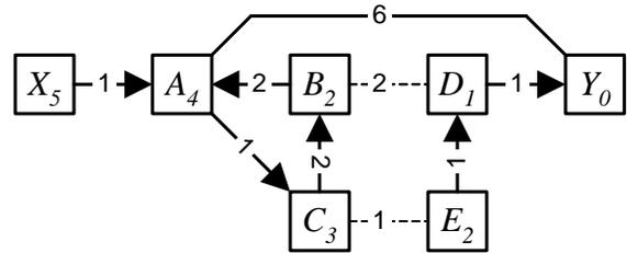
Figure 2—Loop suppressed by exact hop count
