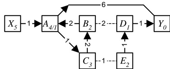
Figure 3—Packet looping in a loop-free network
