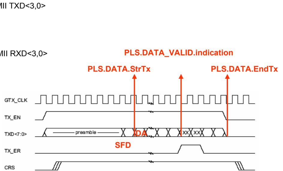
Figure 35-4—Propagating an error within a frame
