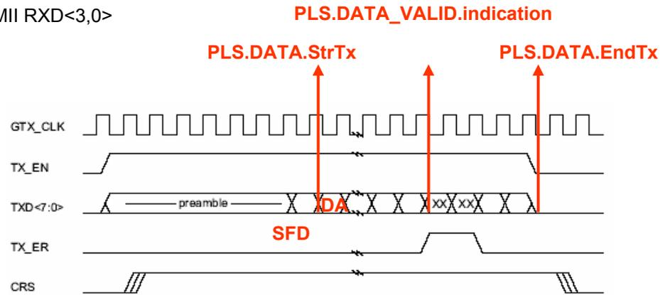
Figure 35-4—Propagating an error within a frame
