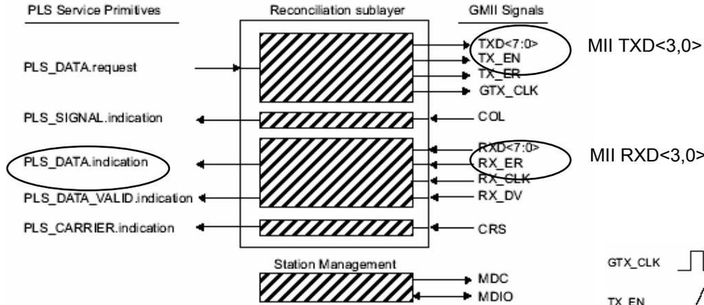
Figure 35-2—Reconciliation Sublayer (RS) inputs and outputs and STA connections to GMII
