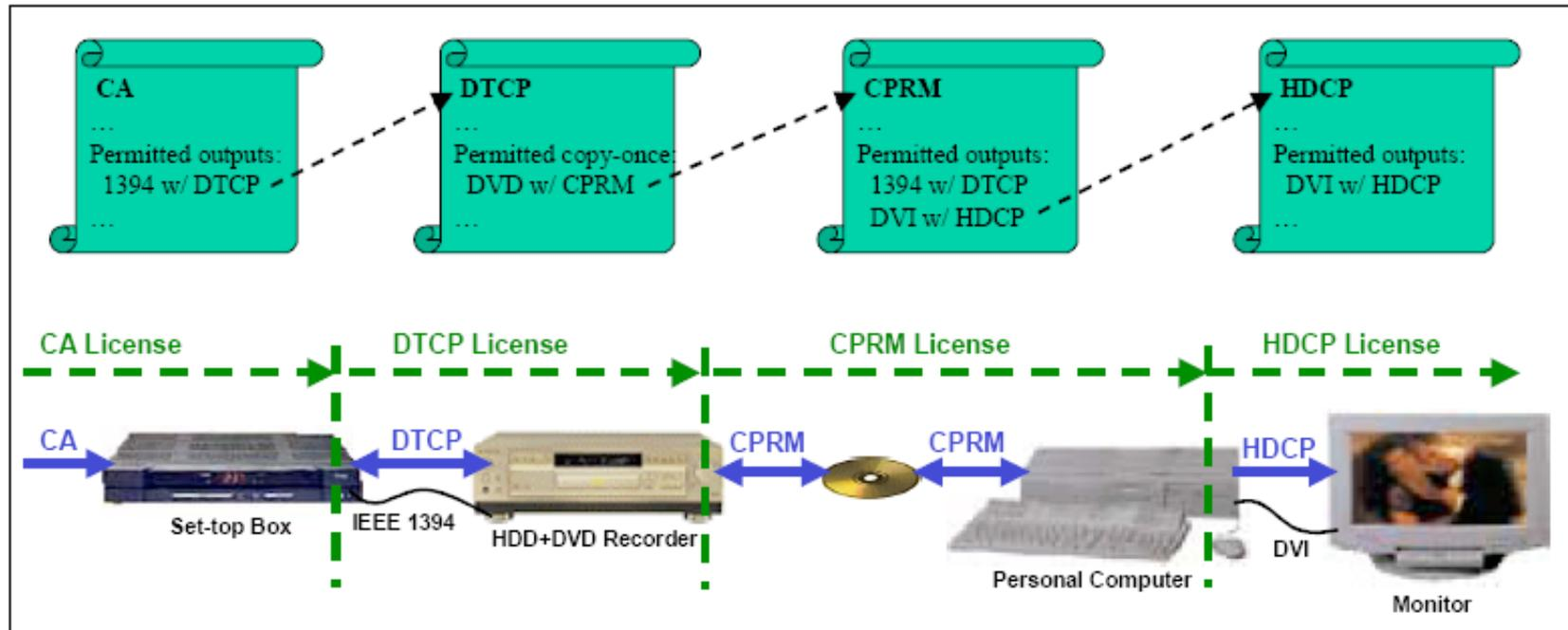
Figure 3: Content protection chain example
