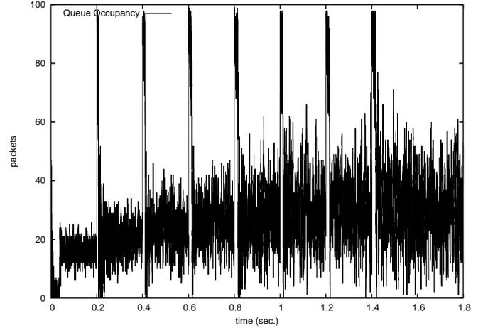
Fig. 2. Queue-size at the buffer attached to a 10Gbps link; no self-increase.
