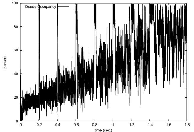
Fig. 3. Queue-sizes under algorithm SI-1. Gentle increase of 10 Mbs/s (top) and aggressive increase of 500 Mbs/s (bottom).
