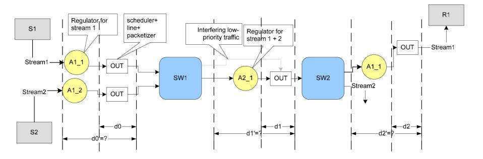
For network with regulators, need to determine values of d0', d1', d2'
