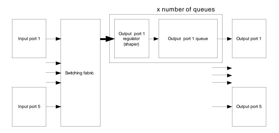
Output port receives measured steam and 3 interfering streams @ 18.75% each = 75% max load
