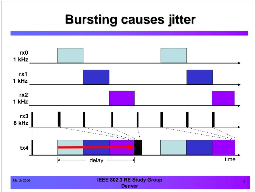
We assume transfers will be cycle-clock based, with an 8 kHz clock.
