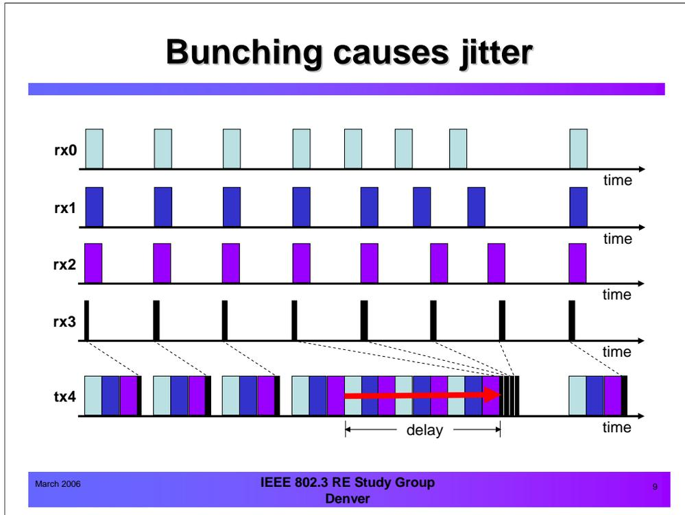
To solve bursting, force sources send at 8 kHz, using only frame lengths (not transmit-frame periodicity) to adjust their transmission rates.
