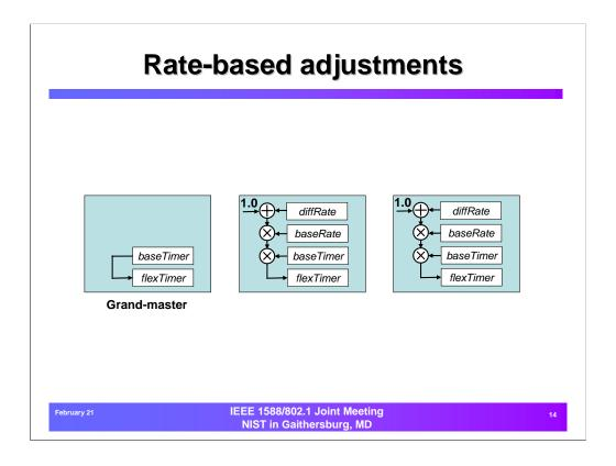
The accumulated rate differences are applied to flexTimers.
