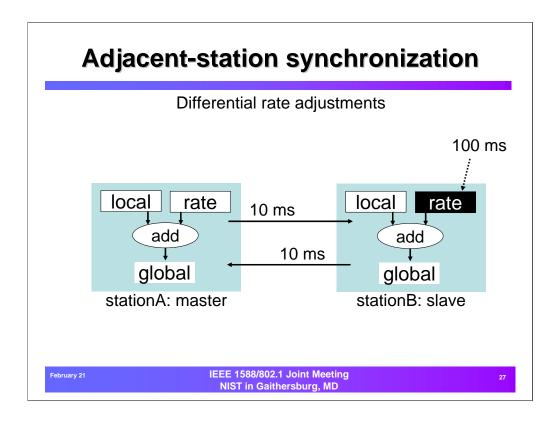
Adjacent-station synchronization is preferrably done less frequently, so that the time-snapshot errors are smaller.
