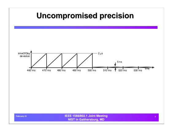
With a 200PPM clock deviation, offset adjustments have limitations.
