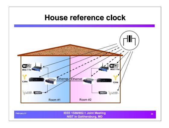
In support of synchronous transfers, all RE devices are assumed to have the same impression of time.
