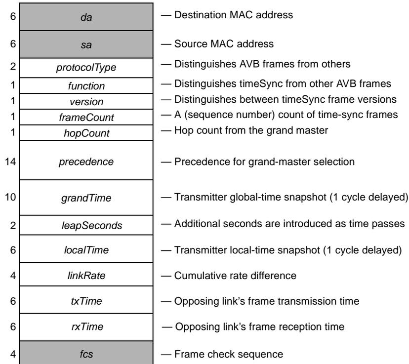
**Figure 6.2—timeSync frame format**
