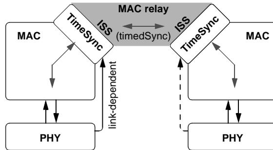
Figure 6.1—MAC-relay interface model
