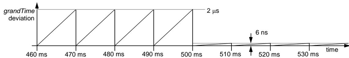
Figure 5.7—Rate-adjustment effects
