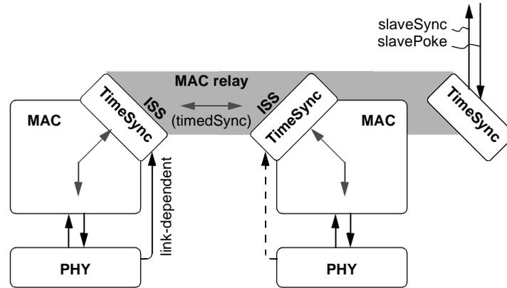
Figure 6.11—Clock-slave interface model
