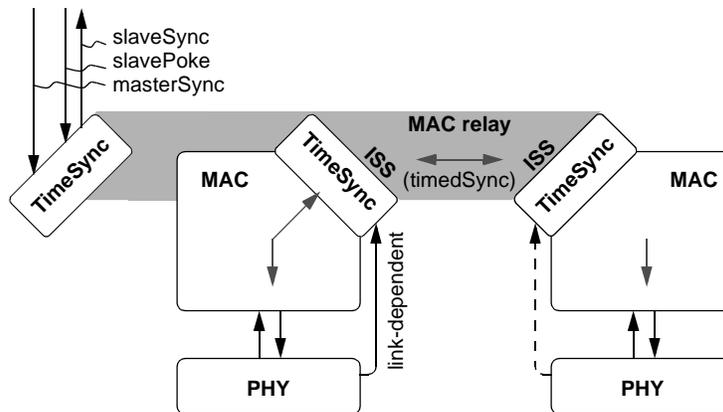
Figure 6.10—Clock-master interface model
