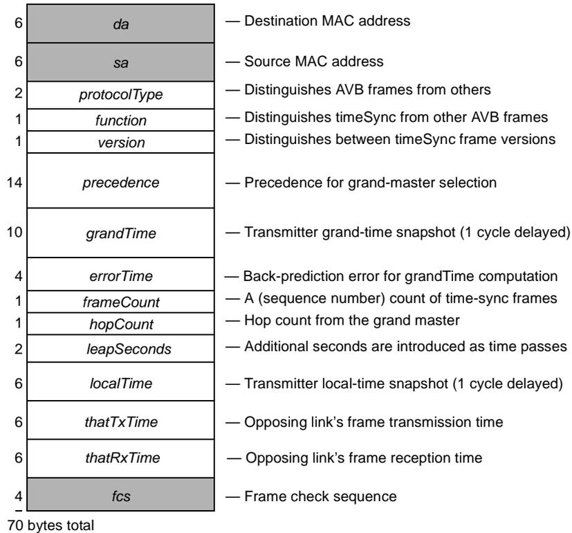
**Figure 7.3—timeSync frame format**
