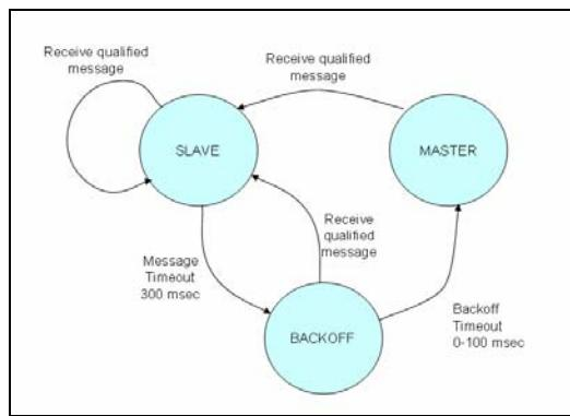
Figure 7-10. Global clock entity state diagram.
