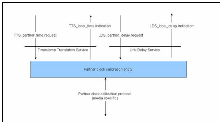
Figure 7-4. TTS and LDS interfaces.
