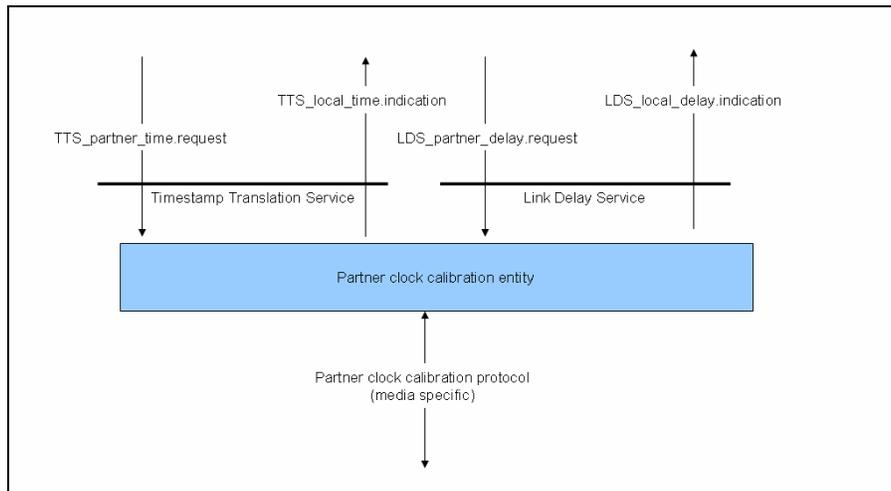
Figure 7-4. TTS and LDS interfaces.
