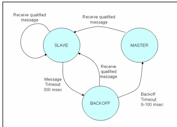
Figure 7-10. Global clock entity state diagram.
