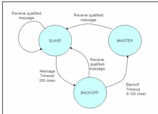
Figure 7-10. Global clock entity state diagram.
