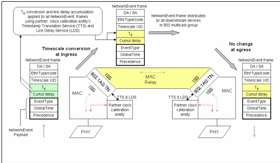
Figure 7-9. Network event frame forwarding model in 802.1D bridging environment.
