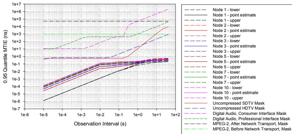
Figure 2 - MTIE results (example from simulation, actual results TBD)
