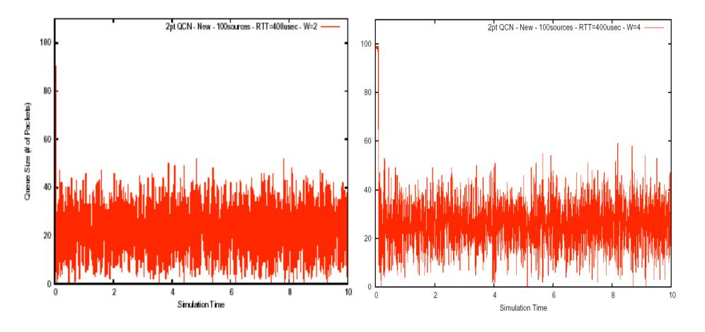
Since Fb = q<sub>off</sub> + wq<sub>delta</sub>, increasing w weights the derivative more and hence leads to less wiggly queues. But because of the springiness of binary increase, even w = 2 performs well at large RTTs.
