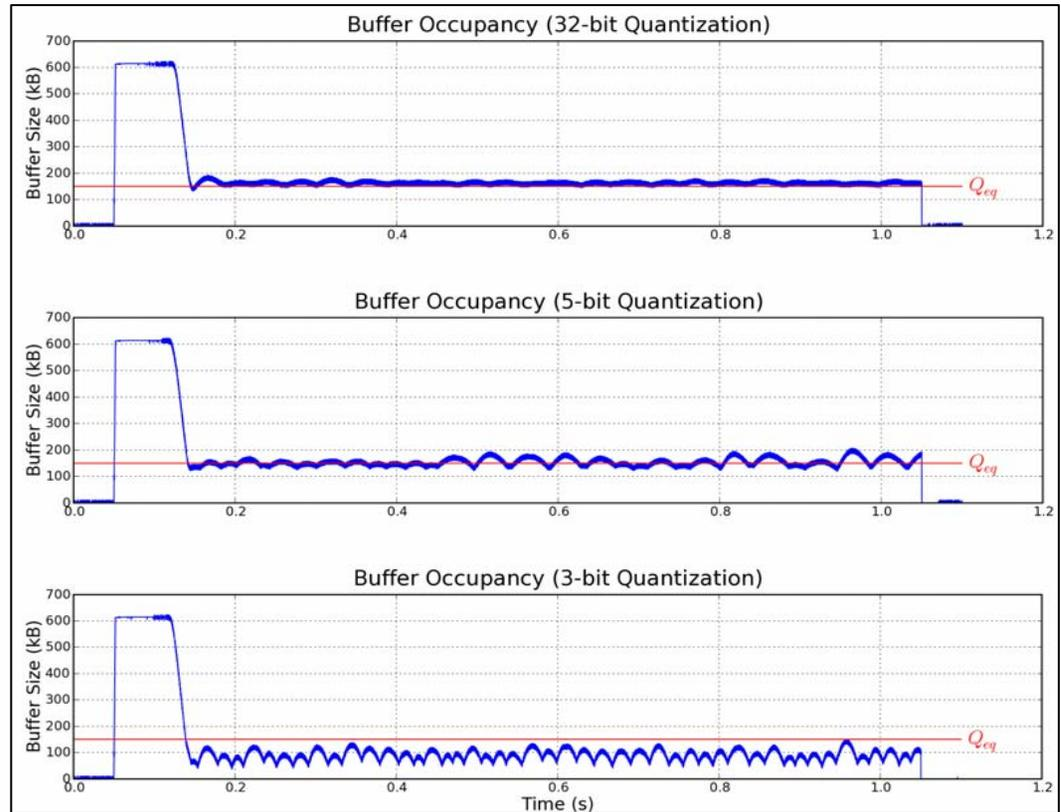
***With Baseline BCN and ONLY varying the degree of quantization of reported Fb signal and no self increase, 5 bits of quantization achieves reasonable performance.***
