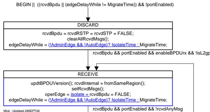
**Figure 2—Changed Port Receive state machine based on correction to 802.1ah**
