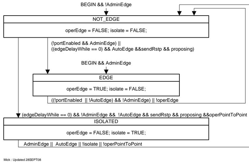
**Figure 1—Replacement Bridge Detection state machine**
