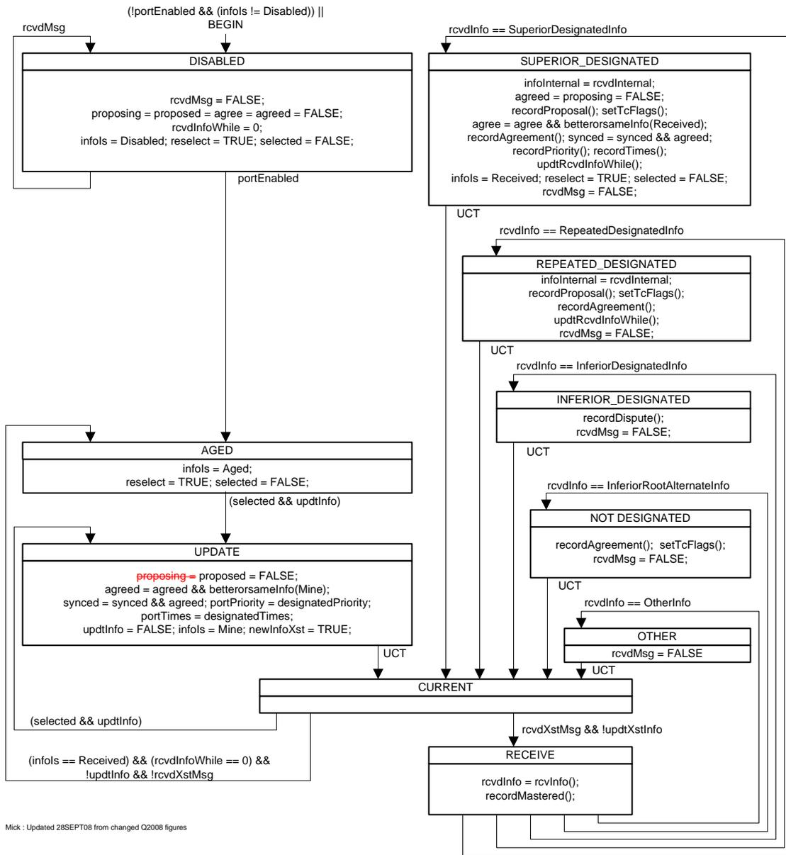
Figure 4—Changed Port Information state machine (change from 802.1Q-2006)
