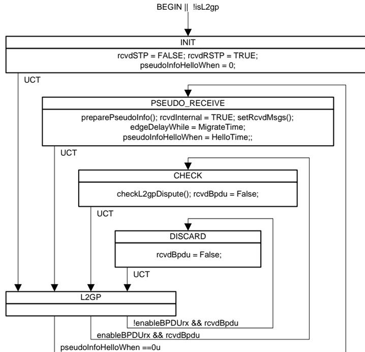
Figure 3—L2 Gateway Port Receive state machine
